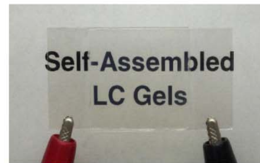
Electric Field ON-State (Transparent)
