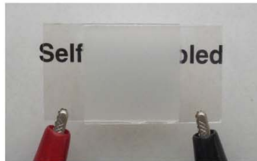
Electric Field OFF-State (Turbid)
